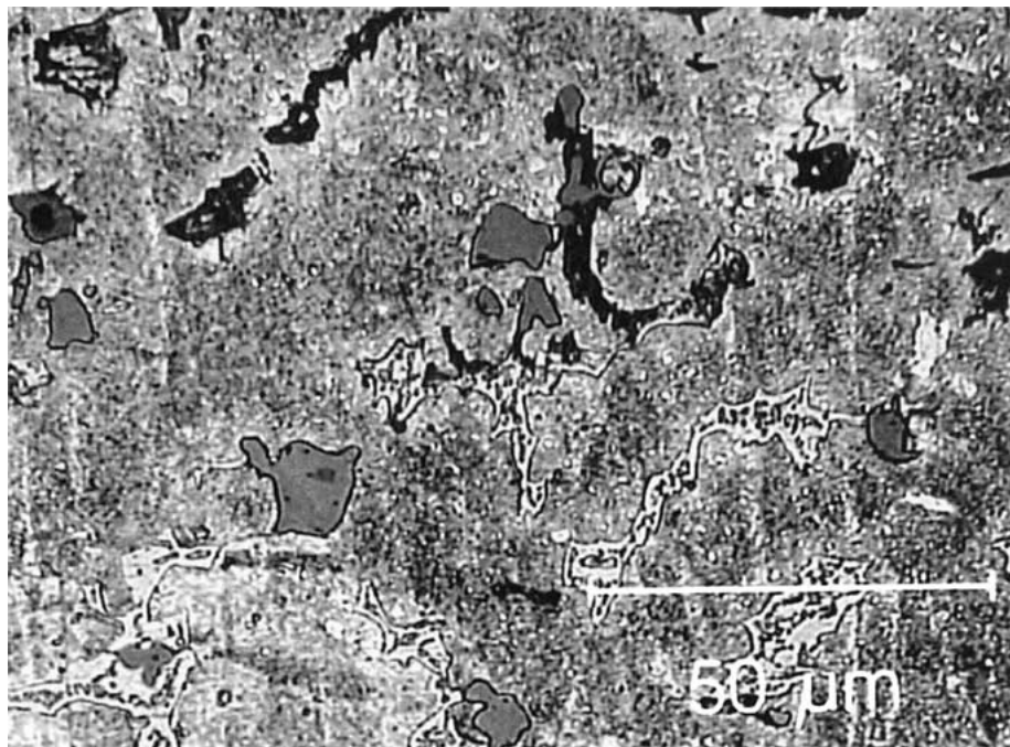
Figure 4 Copper sulphide inclusions (dark grey patches) in the Zun vessel 1B, etched with \text{FeCl}_3/\text{HCl} /ethanol.
